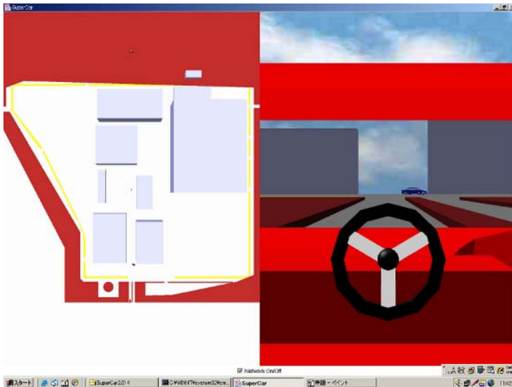
Fig. 2. Double-paned driving simulator window showing exocentric (left, bird's eye) and egocentric (right, driver's perspective) views. (Originally developed by Hideto Shimizu.)
