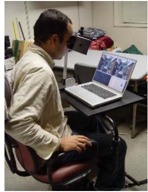
(c) Stereographic viewer on the \mathcal{S}_{\text{hair}}^e desk, used to fuse dynamic stereograms on the laptop.
