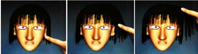
Fig. 8.2. Changes when the robot's hair is stroked from the ends to the roots
